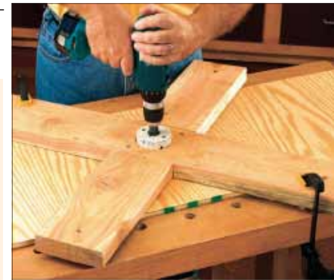
When drilling the 2-1/2-in. center hole, clamp the mounting support firmly to the work surface to prevent the torque from the hole saw from spinning the assembly.
