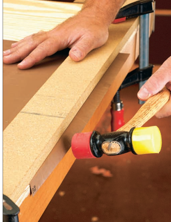
When forming the copper, gently and repeatedly work down the length of the bend, gradually creating the 9/16-in. edge for the overhang.
